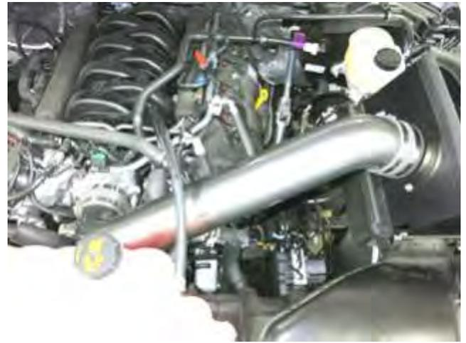
h. Install intake tube at throttle body first, then at air filter tube position in couplers for best fit, then secure by tightening hose clamps. Secure heat shield using factory clips at this point.
