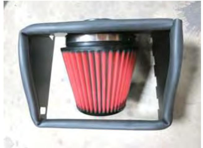
d. Install and secure a filter to a filter adapter using the provided large hose clamp.
