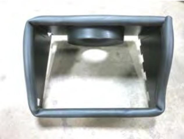
c. Install large edge trim onto top of heat shield, start from a corner, working around unsecured.
