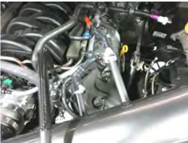
i. Connect factory EVAP and crank case vent connections to the intake tube.
